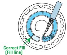
2. Do not overfill the disk. If the disk is overfilled, sample water will flow out of the overflow hole in the center of the disk. The disk is not leaking. Dry the disk and run the test.
