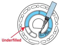
4. Do not introduce air bubbles into the disk. The reagent chambers will not fill entirely and results will be inaccurate. As soon as a bubble starts to form, pull back on the plunger to draw the bubble out of the disk. Begin the filling process again.
