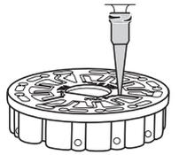
1. Fill the disk using slow, even pressure. The sample water will fill the spaces between the baffles in a counterclockwise order. Each space will fill from the bottom to the top. Sample water should be added until the sample water in the fourth chamber fills **to the top** of the chamber slightly past the embossed fill line. It is OK to fill slightly past the fill line.
