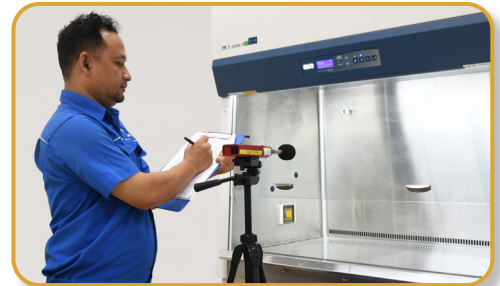
Noise Level Test
