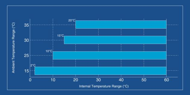
The iTherm CH25 provides temperature control from 15°C below ambient to 60°C, & the lowest achievable temperature is up to 2°C.
