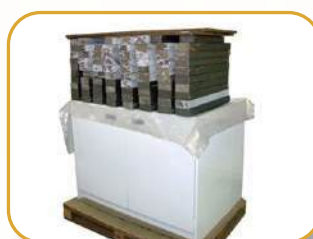
Actual photo during Cabinet Load Testing
