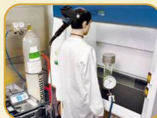
Tracer Gas (SF 6 ) Containment Test
